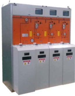
RMC Series Up to 6 feeders with common tank Sf6 Gas Insulation and VI interruption Circuit Breaker and Switch combination 12 ~ 27kV 630A 20/25kA 125 BIL
