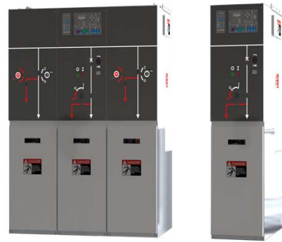
RM Series Extensible Modular type Sf6 Gas Insulation and VI interruption Individual Circuit Breaker or Switch combination 12 ~ 27kV 630/1250A 20/25kA 125 BIL
