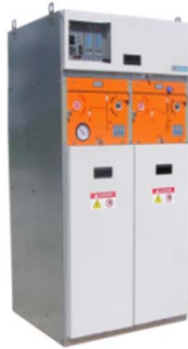
RMF Series Up to 6 feeders with common tank Sf6 Gas Insulation and interruption Fuse-switch and switch combination 12 ~ 27kV 630A 25kA 125 BIL
