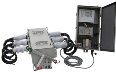
KPS(EPS) series SF 6 gas Load Break Switch 12kV~38kV 630A 25kA 70kV 170 BIL DSP, μ-processor control FRTU function
