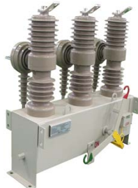
MPS MPS Series Solid Load Break Switch 12~24kV 630A 12.5kA 150 BIL DSP, μ-processor control FRTU function
